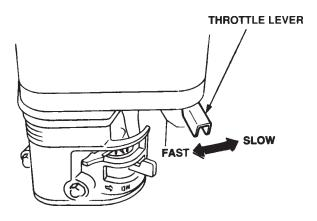
Figure 12. Throttle Lever
